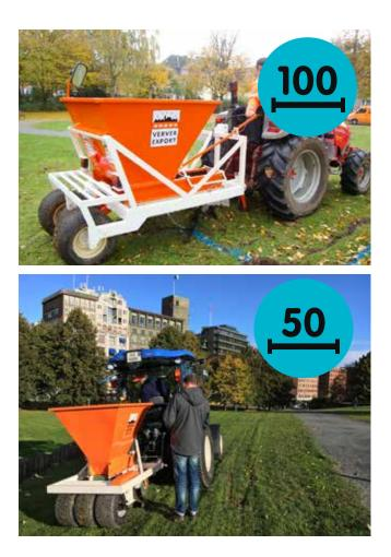
We plant concepts with only dahlias or a mixture of summer bulbs with the planting machine. This involves tilling and planting in one pass at a working width of 100 cm.
