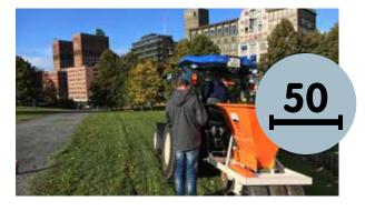
**50 cm planting machine:** plants bulbs across a width of half a metre. Suitable for verges where the operating width in the grass is less than one metre. Or if you want to create long strips but have a more limited budget.
