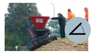
**Embankment Planter:** this machine can plant on a slope with a maximum angle of 30 to 35 degrees. This machine is equipped with caterpillar tracks and an extra planting foot for even planting.
