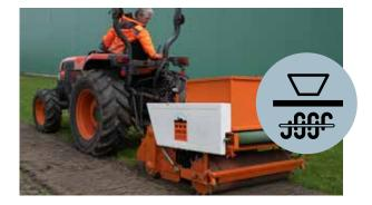
**Roto Planter:** this machine plants across a width of one metre and can rotavate, plant and roll in a single run. Particularly suitable for less heavy soil types. For use with spring-flowering and summer-flowering bulbs.
