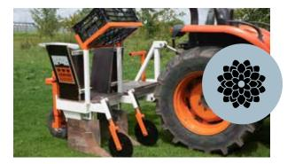
**Dahlia Planter:** a double City Planter whereby the tubers are manually thrown into the trough and planted in 2 rows. There is no roller or other levelling equipment attached to the machine because the soil needs remain airy. Not possible under grass: the soil needs to be rotavated first.
